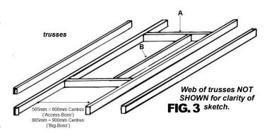
nailed in square. Now cut and nail the third trimmer ('B') to form the width of 770mm in between. Smaller hatches can be manufactured at extra cost or refer to the 'Access-Boss™' series).
